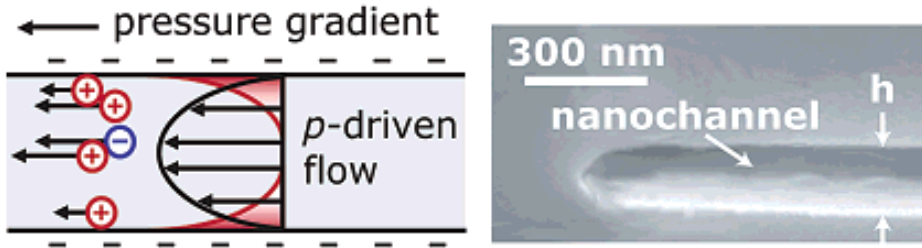
Figure 4 Schematic illustration of electrokinetic effects in nanochannel. Left: a pressure-driven flow carries counter-ions within the double layer, producing a streaming current. Right: Side view of a 200-nm-high silica nanochannel, imaged by scanning electron microscopy.[25]
